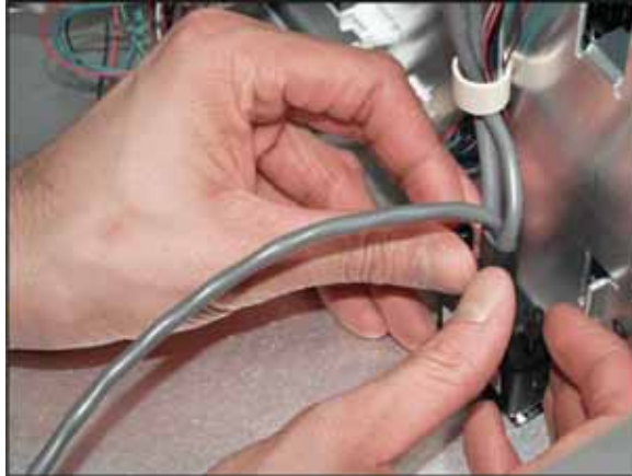
Figure 5-28 LPS Communication Harness
