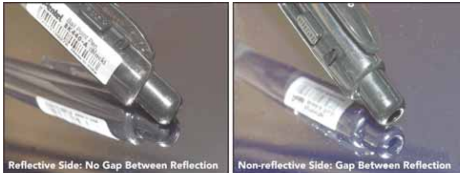
Figure 5-73 Installing Cold Mirror
