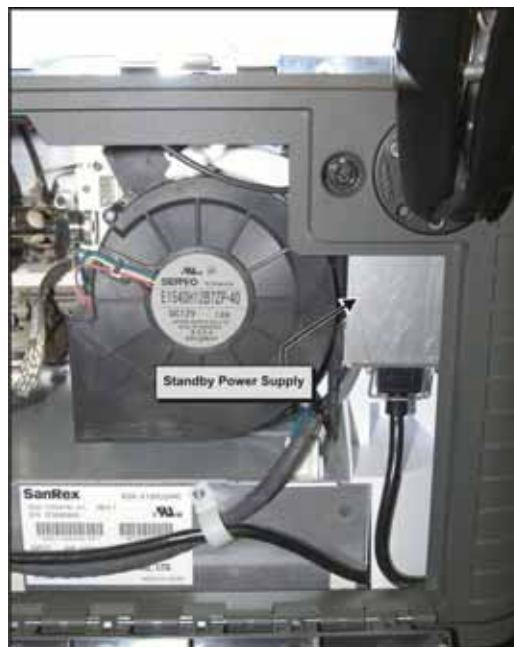
Figure 5-23 Standby Power Supply
